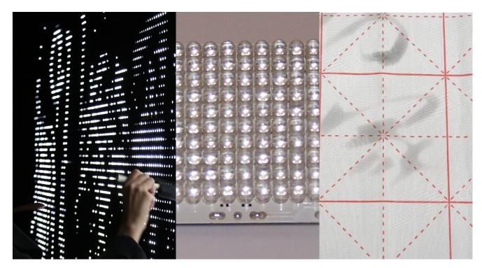
and the similar reaction of the cloth material and electronic circuit, when writing with a damned brush on the crafted LED panel, the brush path will light up, and will fade away as the water dies. This device is designed to encourage a magical experience for the audience to create a piece of art with electronics.
